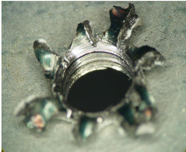
Fig. 14 - The appearance of the produced thread by the sample ZnMg marked M[20]
