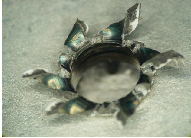
Fig. 13 - The appearance of produced hole by the sample ZnMg marked M[20]
