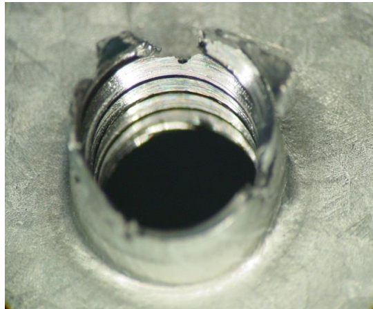
Fig. 12 - The appearance of the produced thread by the sample ZnAl, marked T[20]
