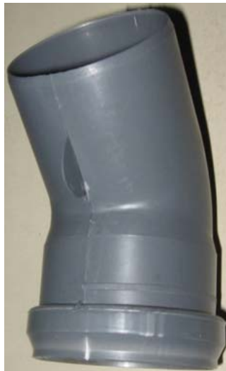
Fig.8 – Noticeable welding lines
