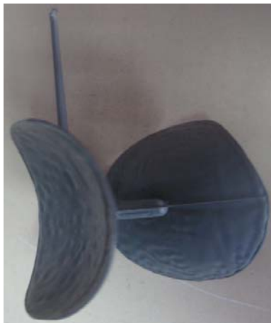
Fig.5 - Short shot error due to dirt in the nozzle
