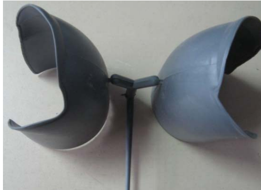
Fig.7 - Short shot errors due to insufficiently heated tool
