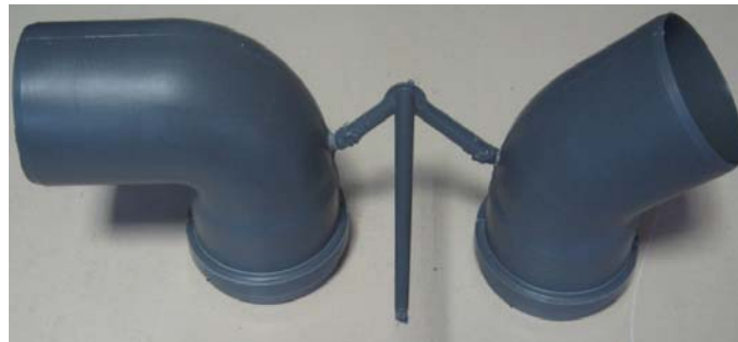
Fig.9 - Pipe fittings injected after FMEA correction actions (no visible errors present)
