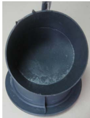
Fig.6 - Overflow error due to high injection pressure
