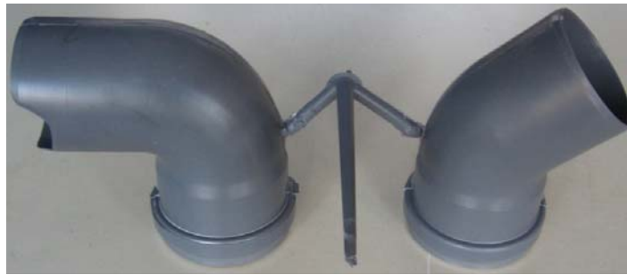
Fig 4. - Short shot error for fitting 75/90° due to unbalanced runner system and low injection pressure
