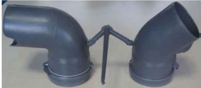
Fig.3 - Overflow error for fitting 75/45° and short shot error for fitting 75/90° due to unbalanced runner system and low clamping force (760kN)
