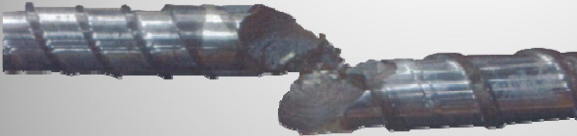
Fig. 1— Typical Wear Pattern in a Single-Screw Extruder
