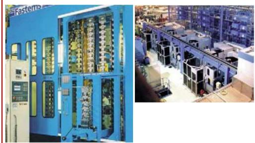
[Fastems central tool storage \(CTS\) for CNC machine tools](#)
