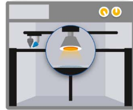
Lamps pass over the surface constantly, the jetted material captures and distributes the heat
