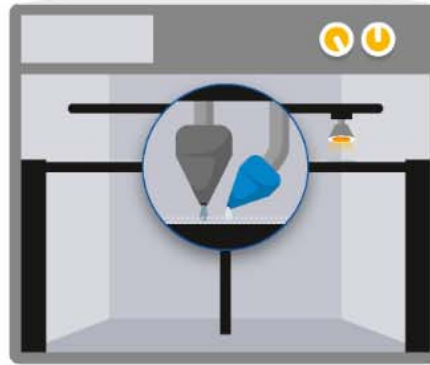
A fusing agent and a detailing agent are jetted to selectively melt powder particles and improve resolution
