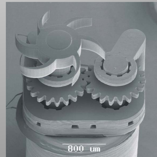
SEM photo of micro turbine The time required for the production of 18 pcs. was approximately 1 hour.
