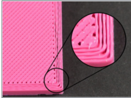
Under-Extrusion
