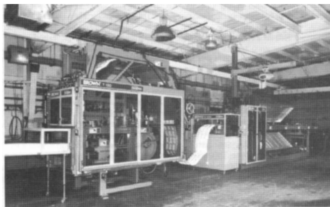
Photo 14.3 Continuous thermoforming machine (Courtesy: Brown Machine)
