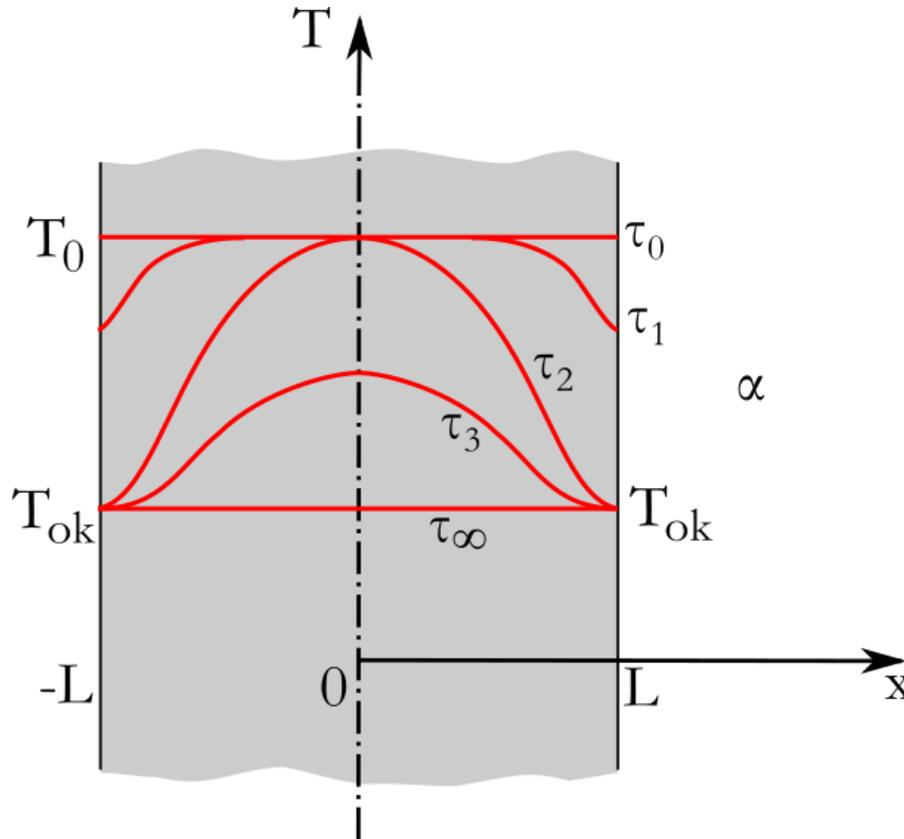
$$\frac{\partial}{\partial x} \left( \lambda \frac{\partial T}{\partial x} \right) = \rho c_p \frac{\partial T}{\partial \tau}$$
